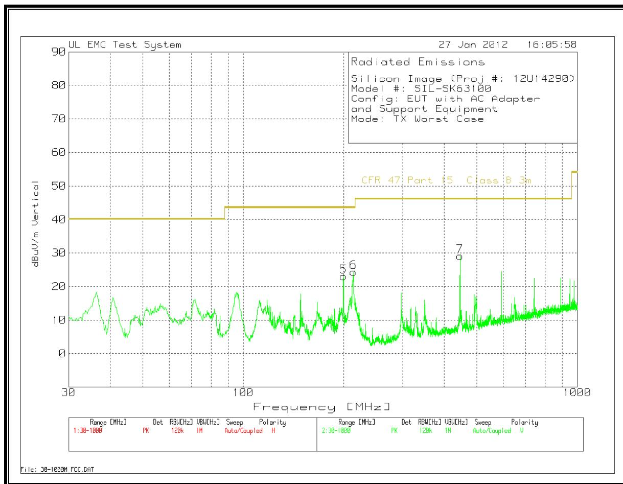
**TX AND RX SPURIOUS EMISSION 30 TO 1000 MHz VERTICAL AND HORIZONTAL DATA**
