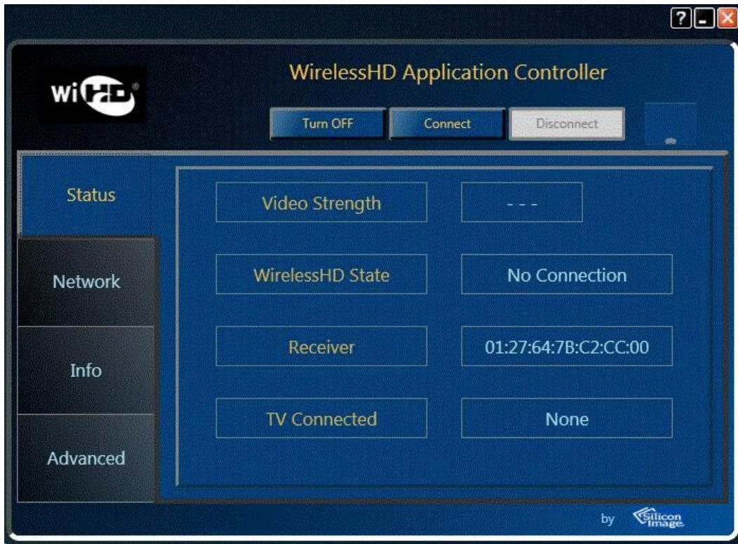
Ensure that the WiHD transmitter is turned on. The left most of the top three buttons will indicate "Turn WiHD OFF" (see screenshot above) when the transmitter is turned on and enabled. If this button indicates "Turn WiHD ON", the transmitter is turned off therefore press this button once and within a couple seconds the button will change its status to "Turn WiHD OFF" and the WirelessHD transmitter will be turned on and
