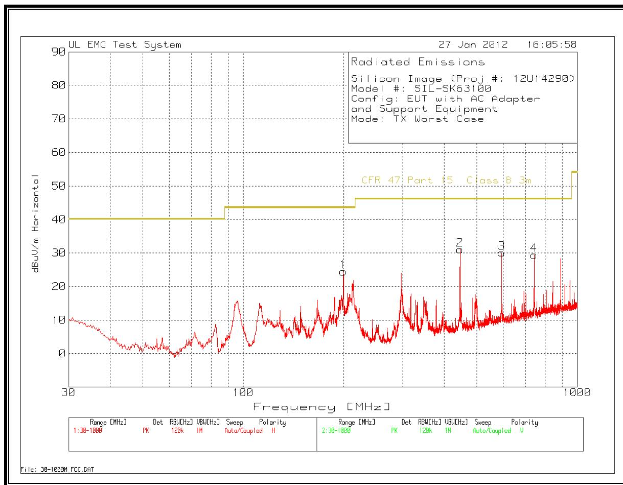
**TX AND RX SPURIOUS EMISSION 30 TO 1000 MHz (VERTICAL PLOT)**
