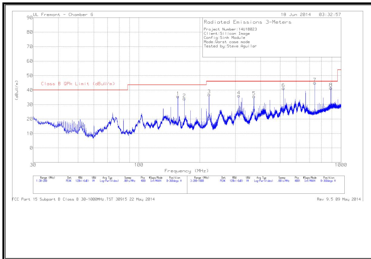
**TX AND RX SPURIOUS EMISSION 30 TO 1000 MHz (VERTICAL PLOT)**
