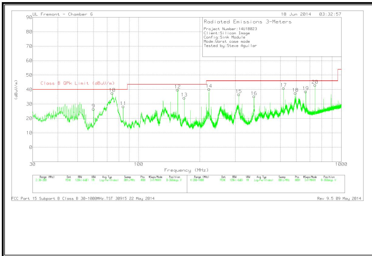
**TX AND RX SPURIOUS EMISSION 30 TO 1000 MHz VERTICAL AND HORIZONTAL DATA**
