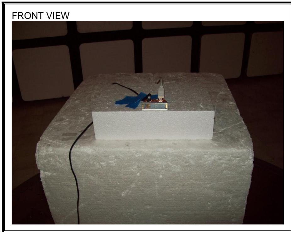
**RADIATED MEASUREMENT ABOVE 1 GHz SETUP**
