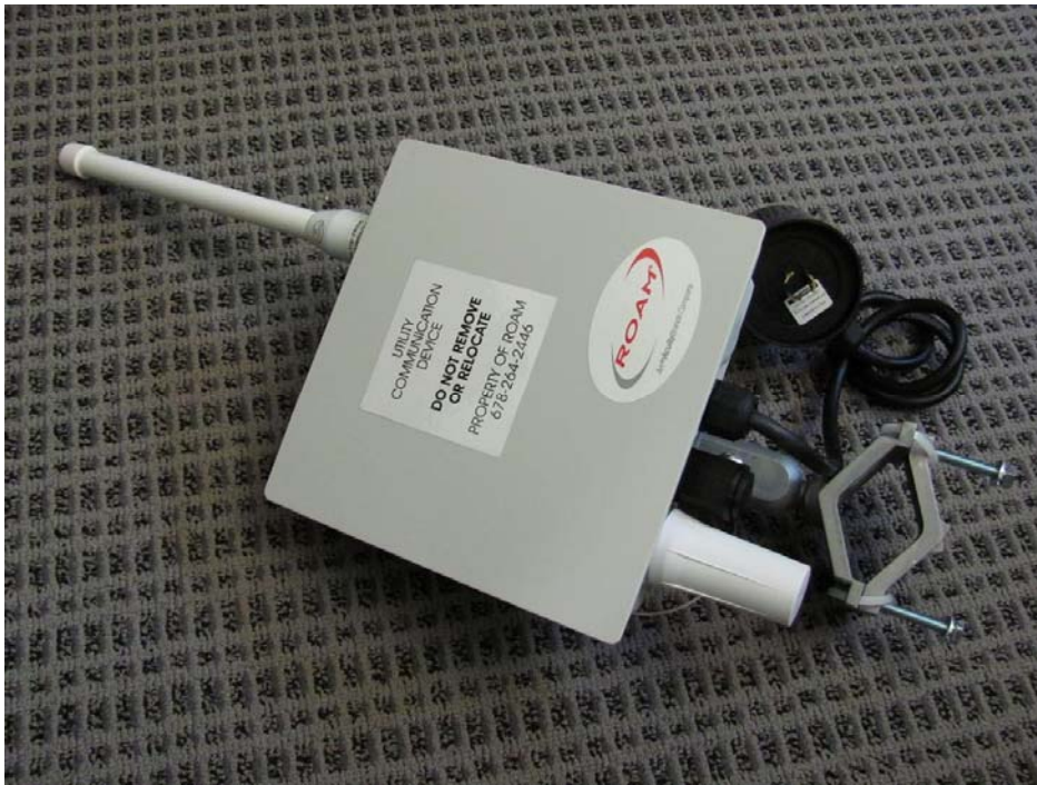
ROAM REG127 gateway contains ROAMMOD0001 radio module 8000-002 variant
