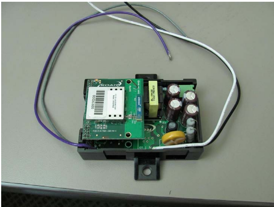
ROAM DCM127 dimming module contains ROAMMOD0001 radio module 8000-004 variant (shown with plastic cover removed).
