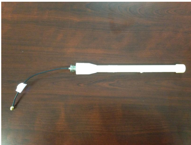
Figure 2. External Monopole, #TQJ-2400D N Male 5 dBi Antenna with reverse pole SMA connector to radio board.
