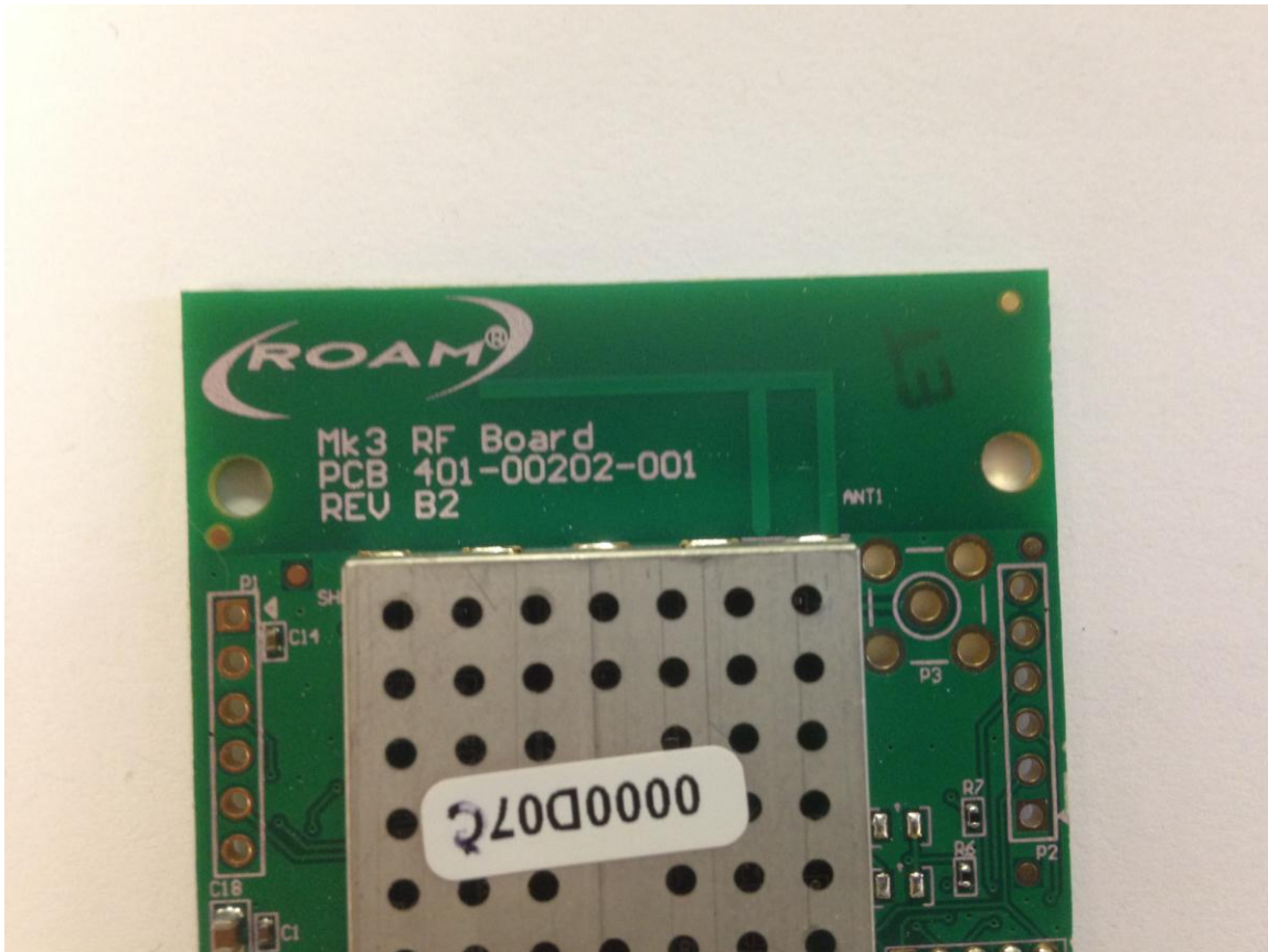
Figure 3. PIFA Trace, Etched on the PCB, 2 dBi Antenna
