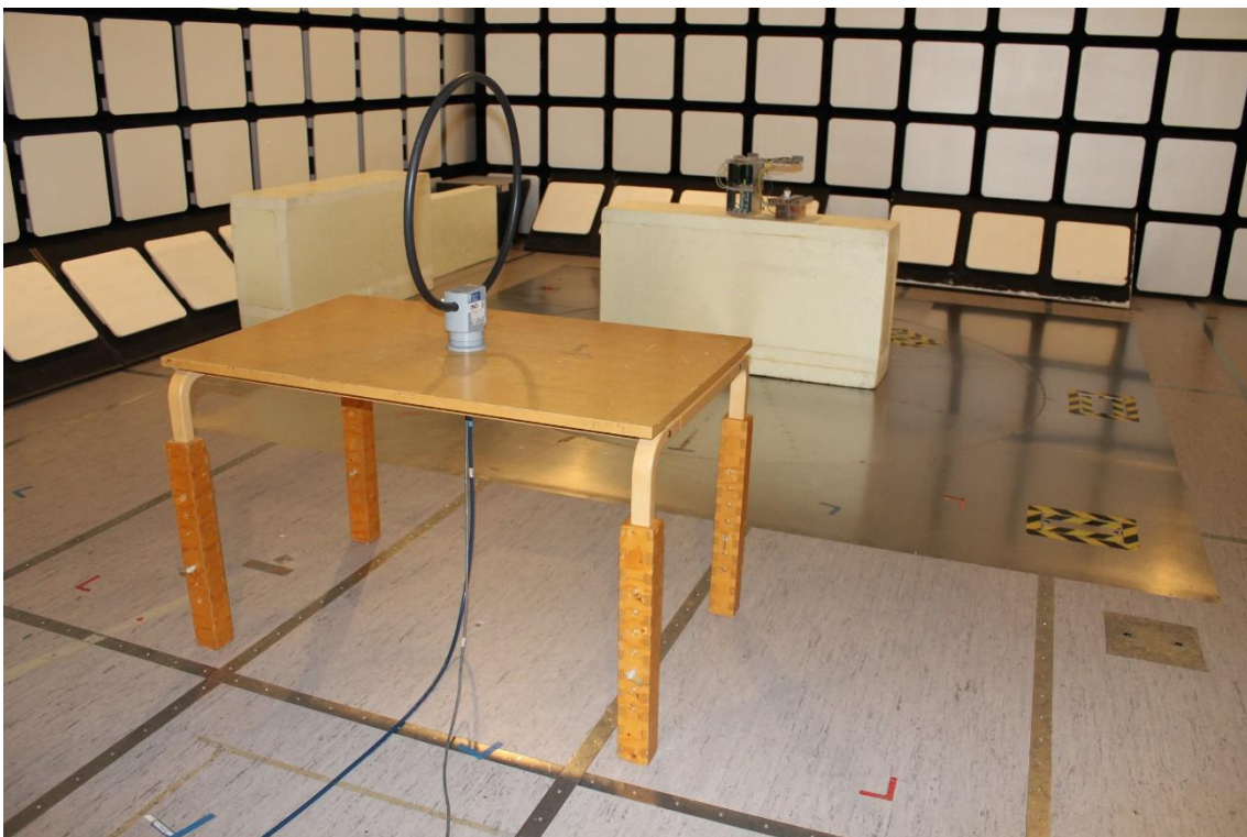
Photograph 6. Radiated Emissions 9 kHz – 30 MHz
