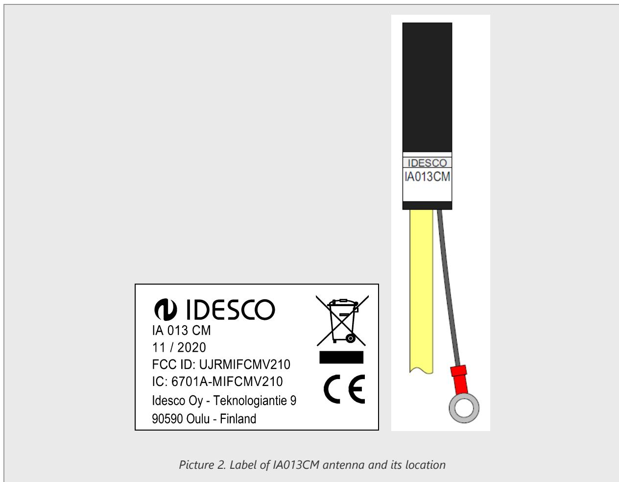
Picture 2. Label of IA013CM antenna and its location
