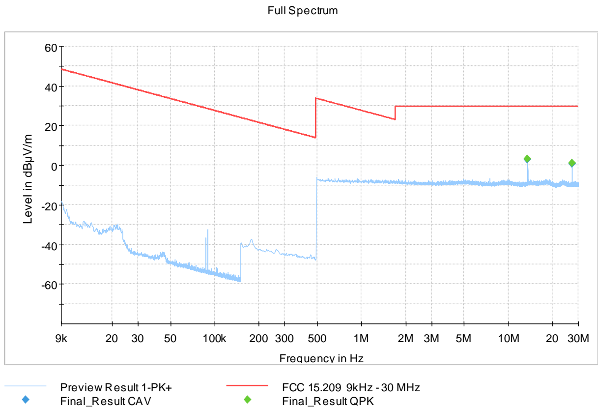
Figure 5. TX radiated emission 9 kHz to 30MHz, Cylinder antenna with TAG
