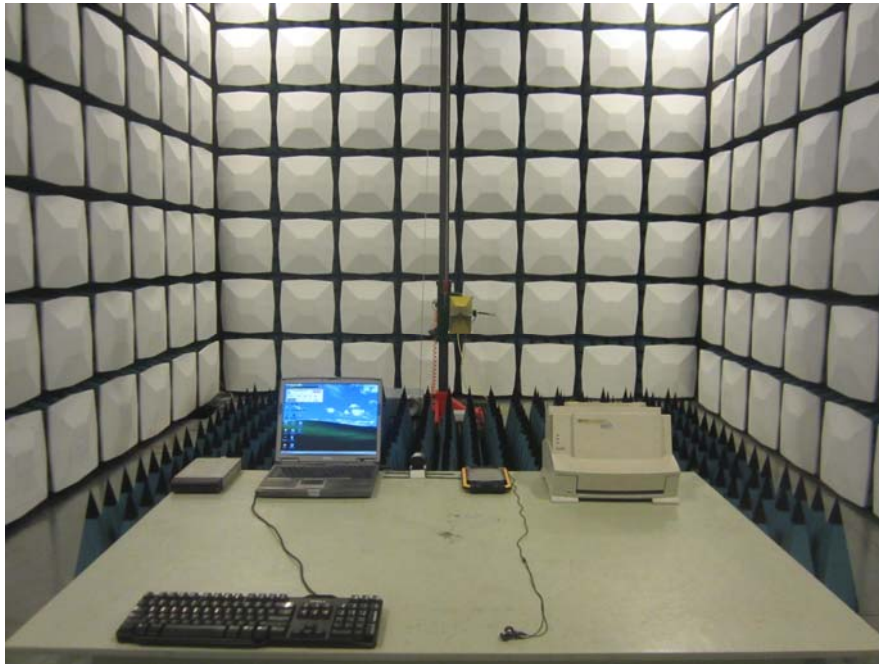
Radiated Emission -Front View (USB Downloading) (Above 1GHz)
