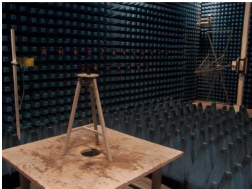
**3. Radiated RF Test (9kHz~30MHz)**
