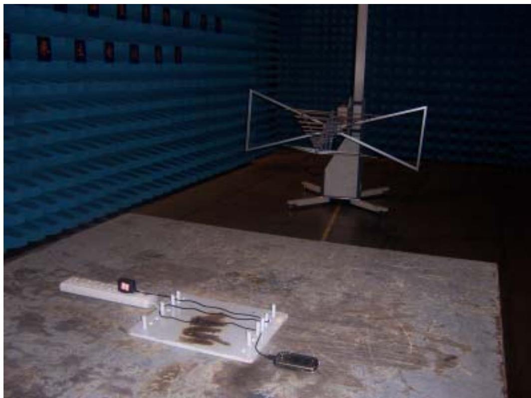
**4. Radiated Emission Test, USB Mode**
