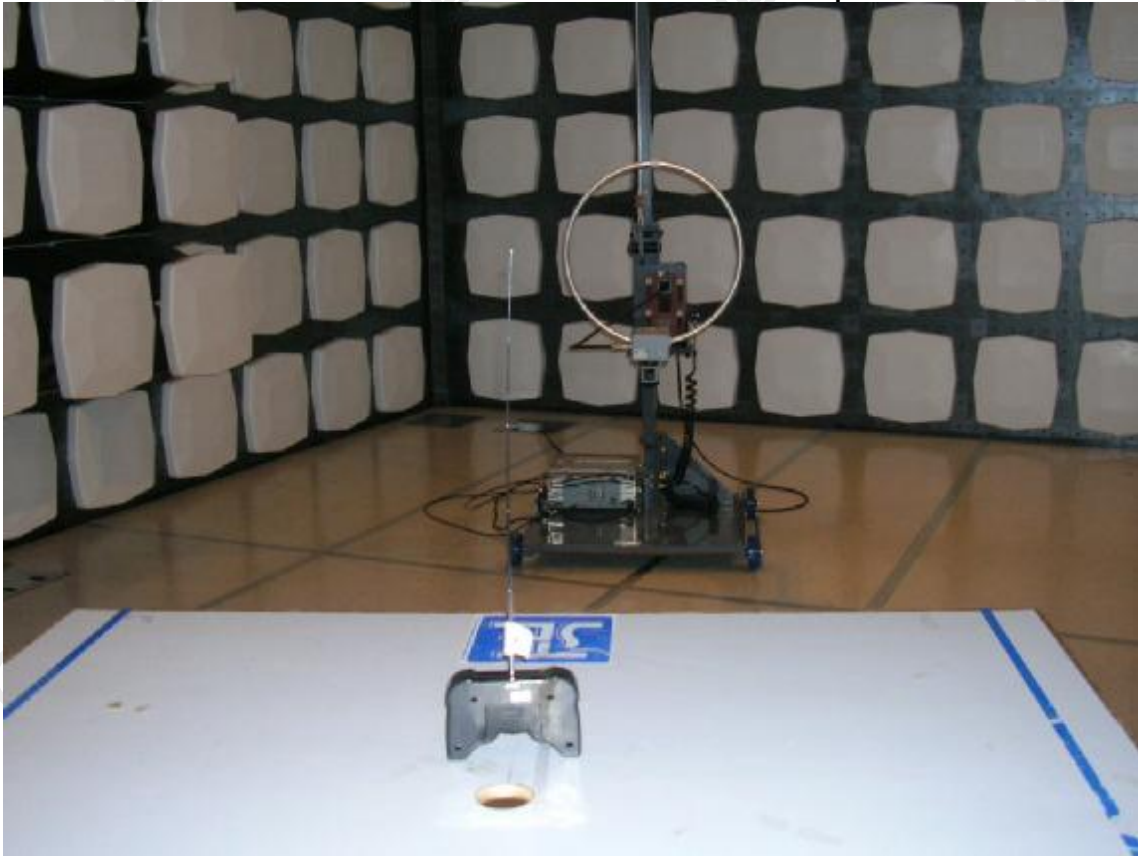
Measurement of Radiated Emission Test Set Up
