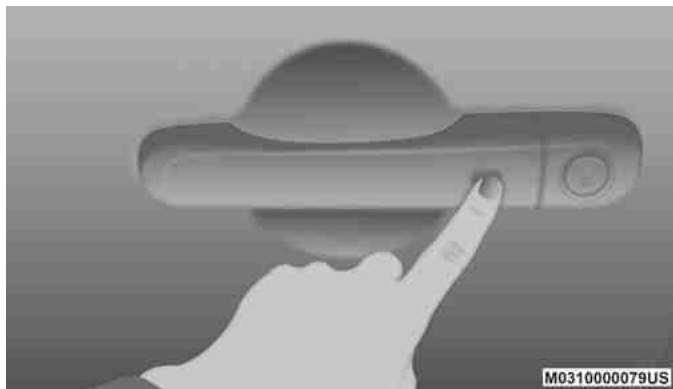
Push The Door Handle Button To Lock
