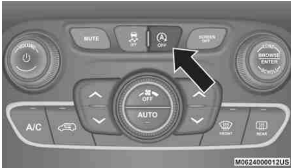
Stop/Start OFF Switch
