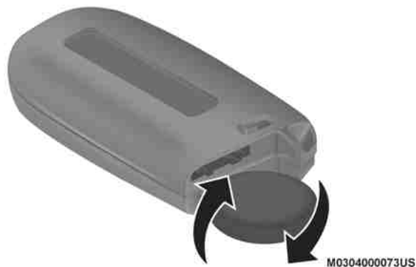
Separating Case With A Coin
