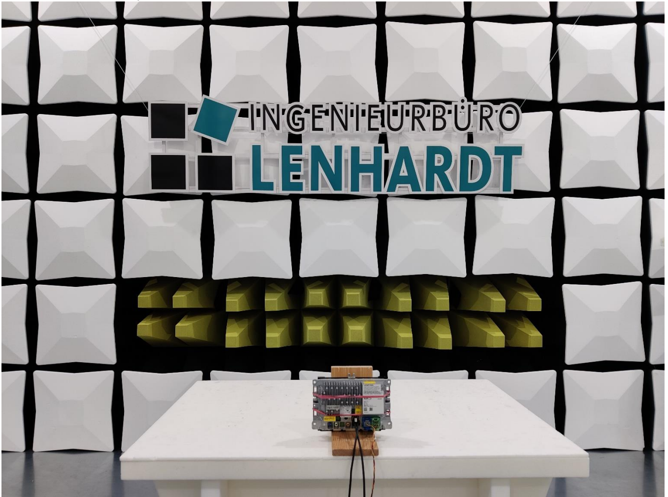
Photo No. 1: Test set-up 8.1, EUT table 0.8 m
