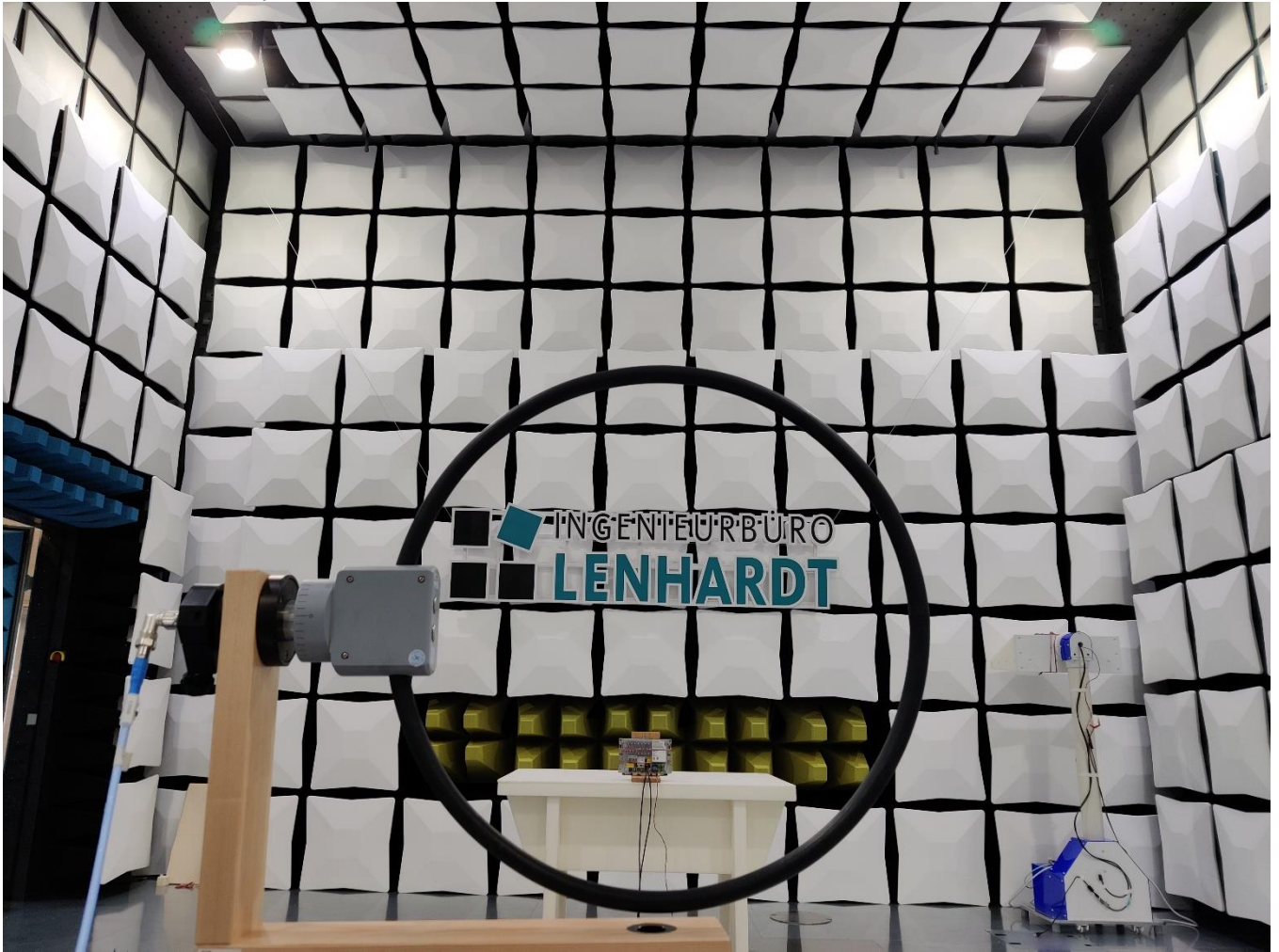
Photo No. 2: Test set-up 8.1, test antenna view
