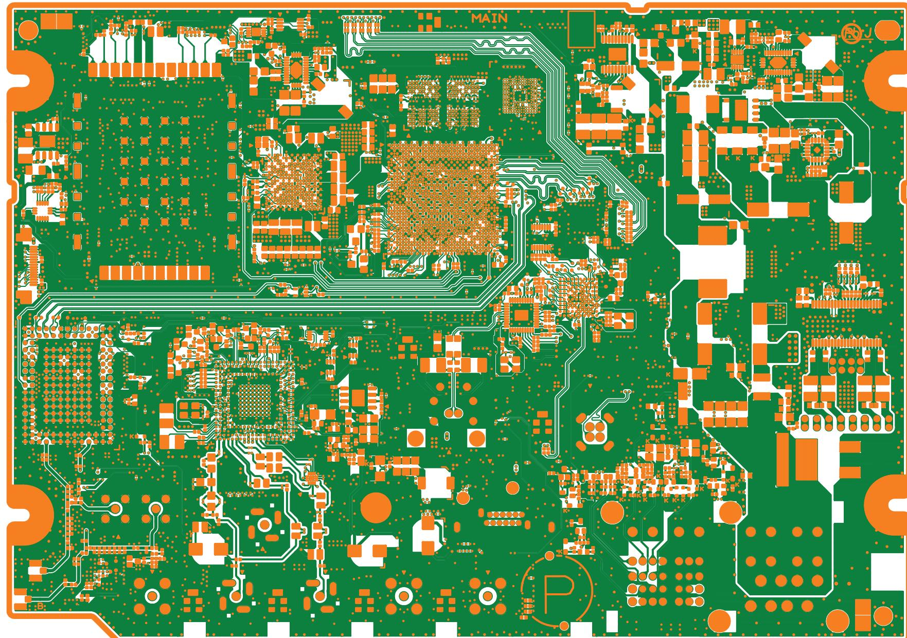
Note: This PCB layout can be shared by all variants. Because PCB and schematic are common to all variants. The variant types are realized by mounting or no-mounting of the components.
