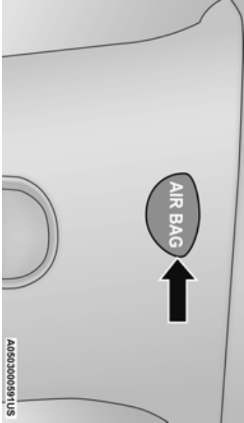
Supplemental Side Air Bag Inflatable Curtain (SABIC)
