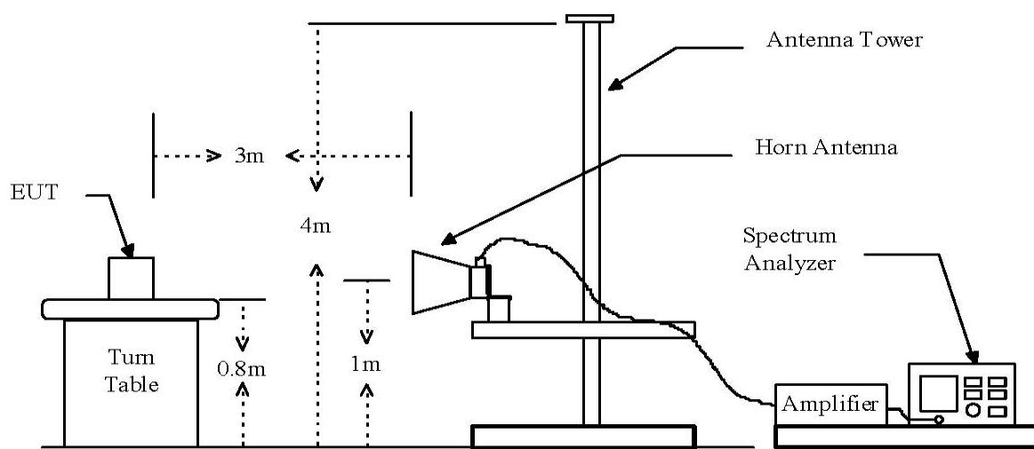
Frequencies measured above 18 GHz configuration
