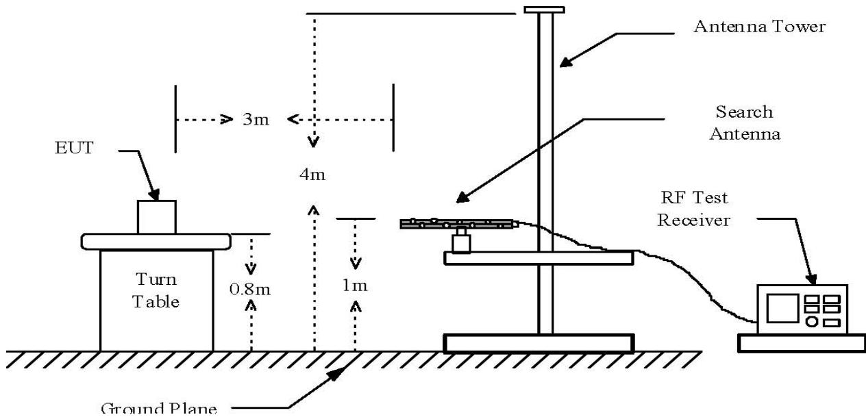
Frequencies measured from 1GHz to 18 GHz configuration
