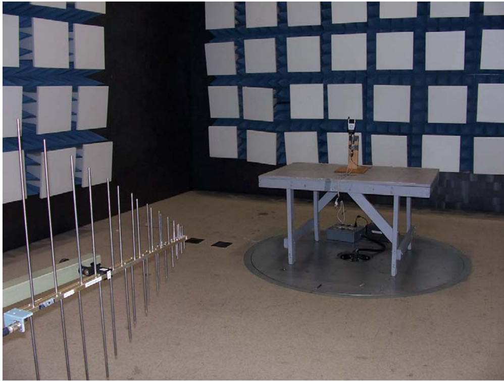
Figure 7 - Photo of Part 15.239 testing set up (Front)
