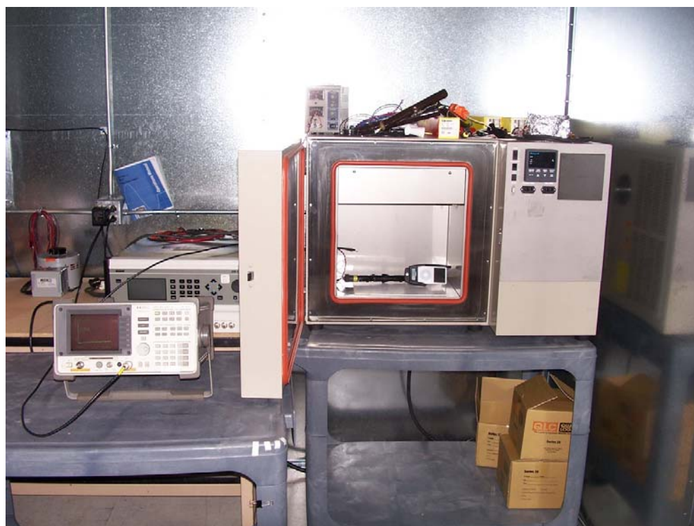
Figure 13 - Photo of test setup for Frequency Stability over Temperature Variations
