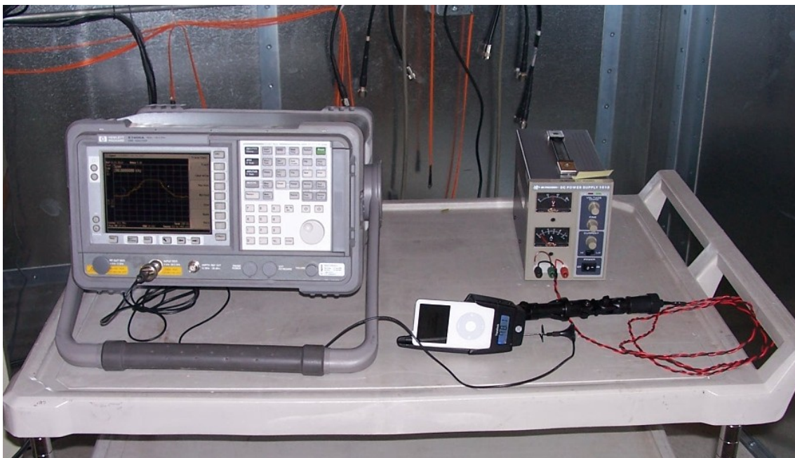
Figure 14 - Photo of test setup for Frequency Stability over Voltage Variations
