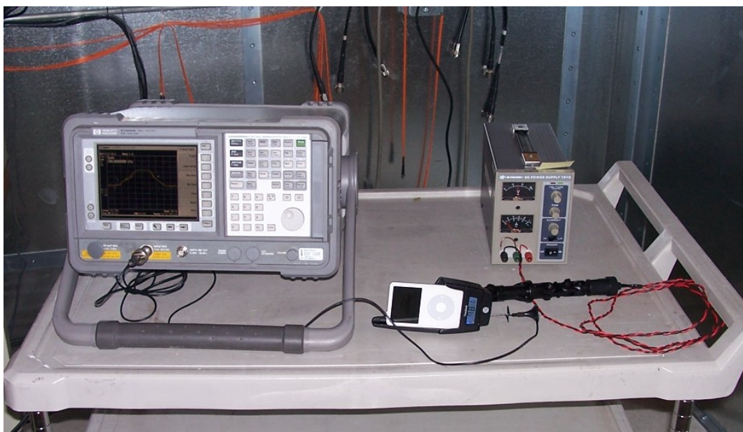
Figure 12 - Photo of 20dB Bandwidth measurement set up
