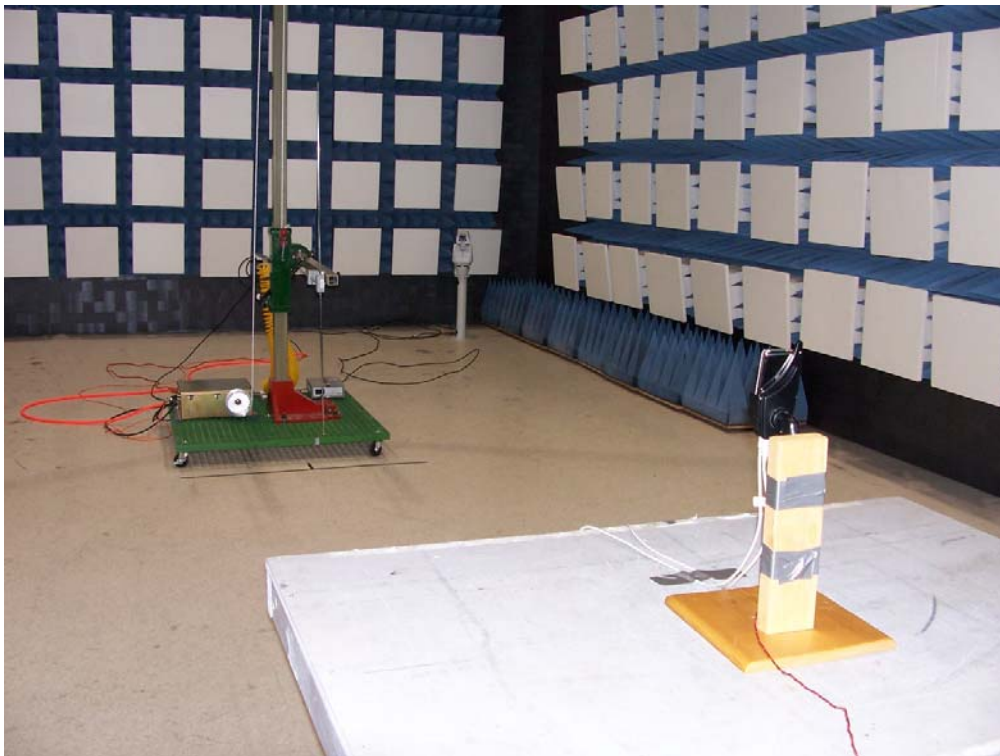
Figure 4 - Photo of Part 15.209 testing set up (Back)
