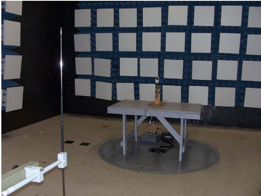
Figure 3 - Photo of Part 15.239 testing set up (Front)
