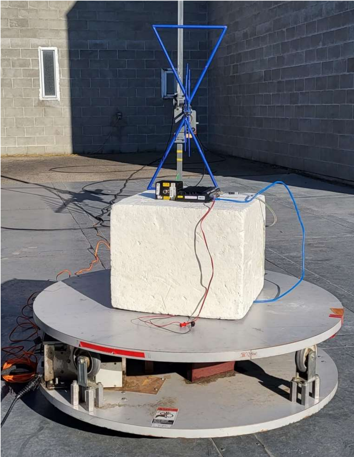
Figure E12.2 – Setup, Radiated Tx Measurements, 30-1000MHz
