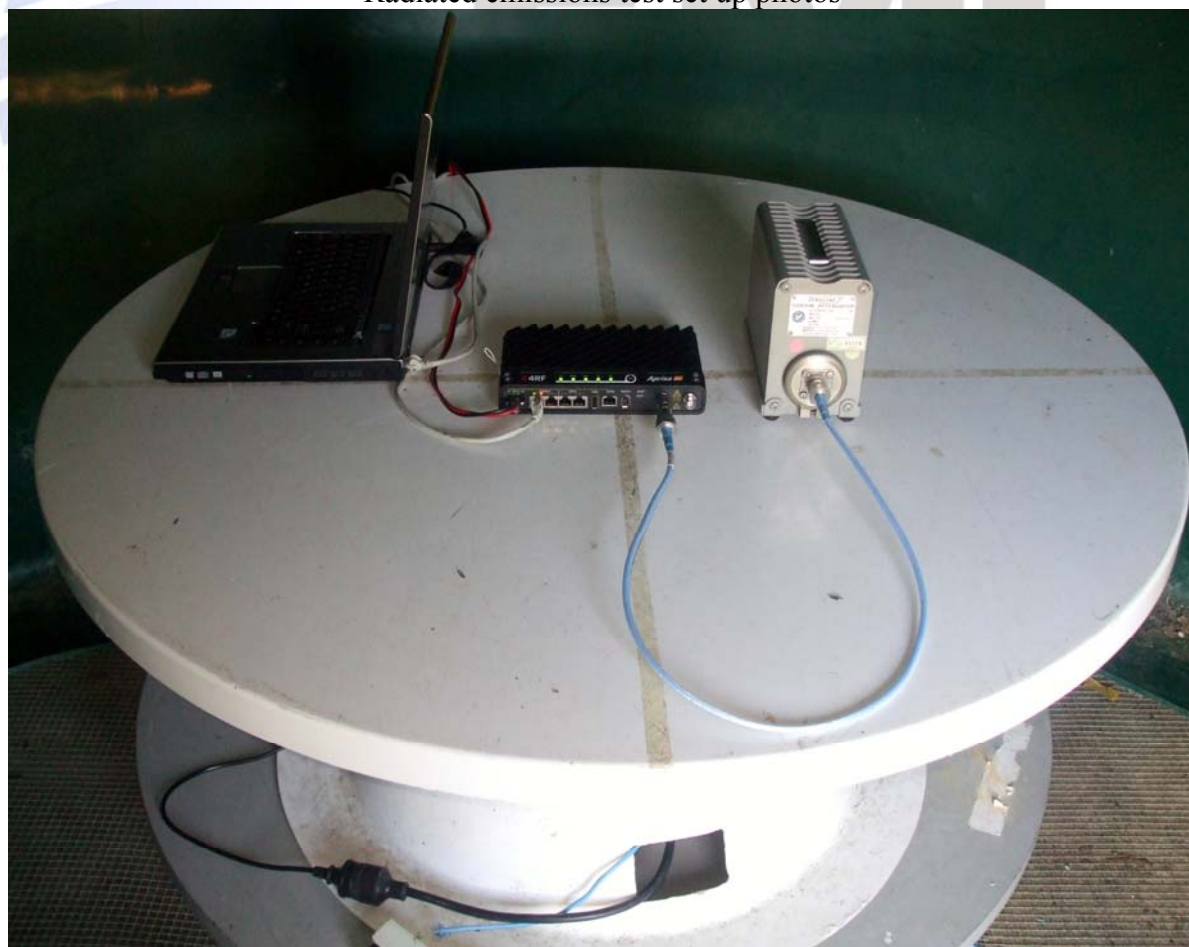
Radiated emissions test set up photos
