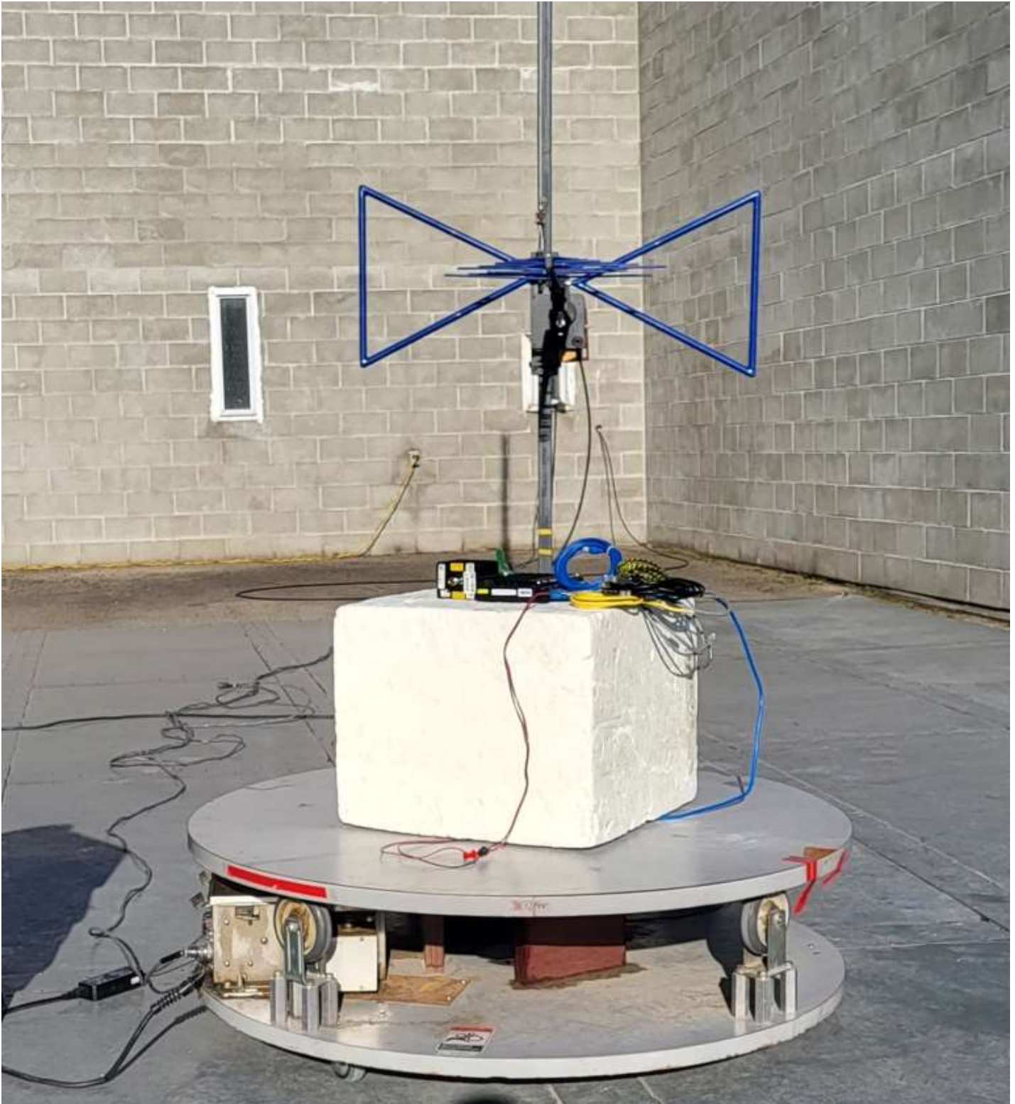
Figure E10.4 – Setup, Radiated Rx Measurements, 30-1000MHz, with Cabling
