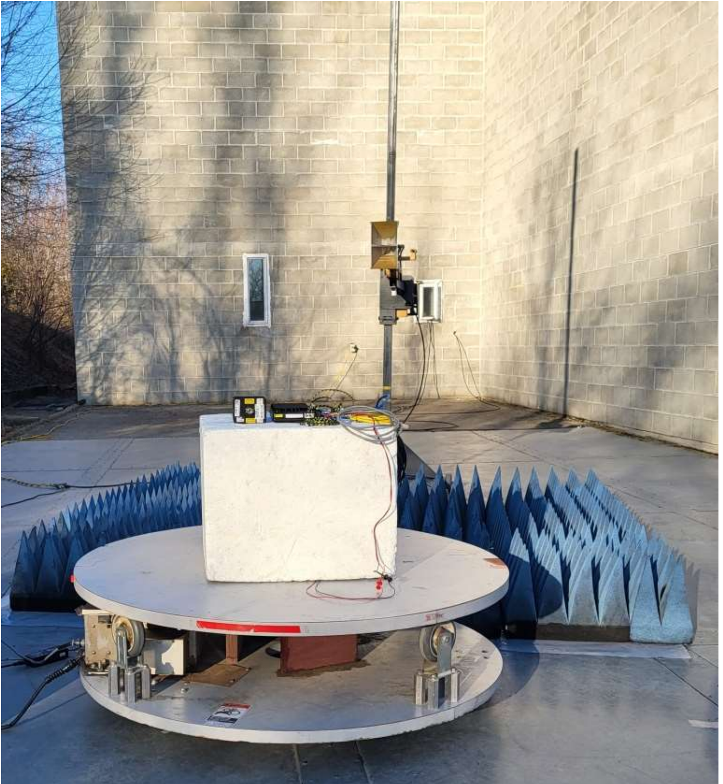
Figure E10.5 – Setup, Radiated Rx Measurements, 1-10GHz, with Cabling
