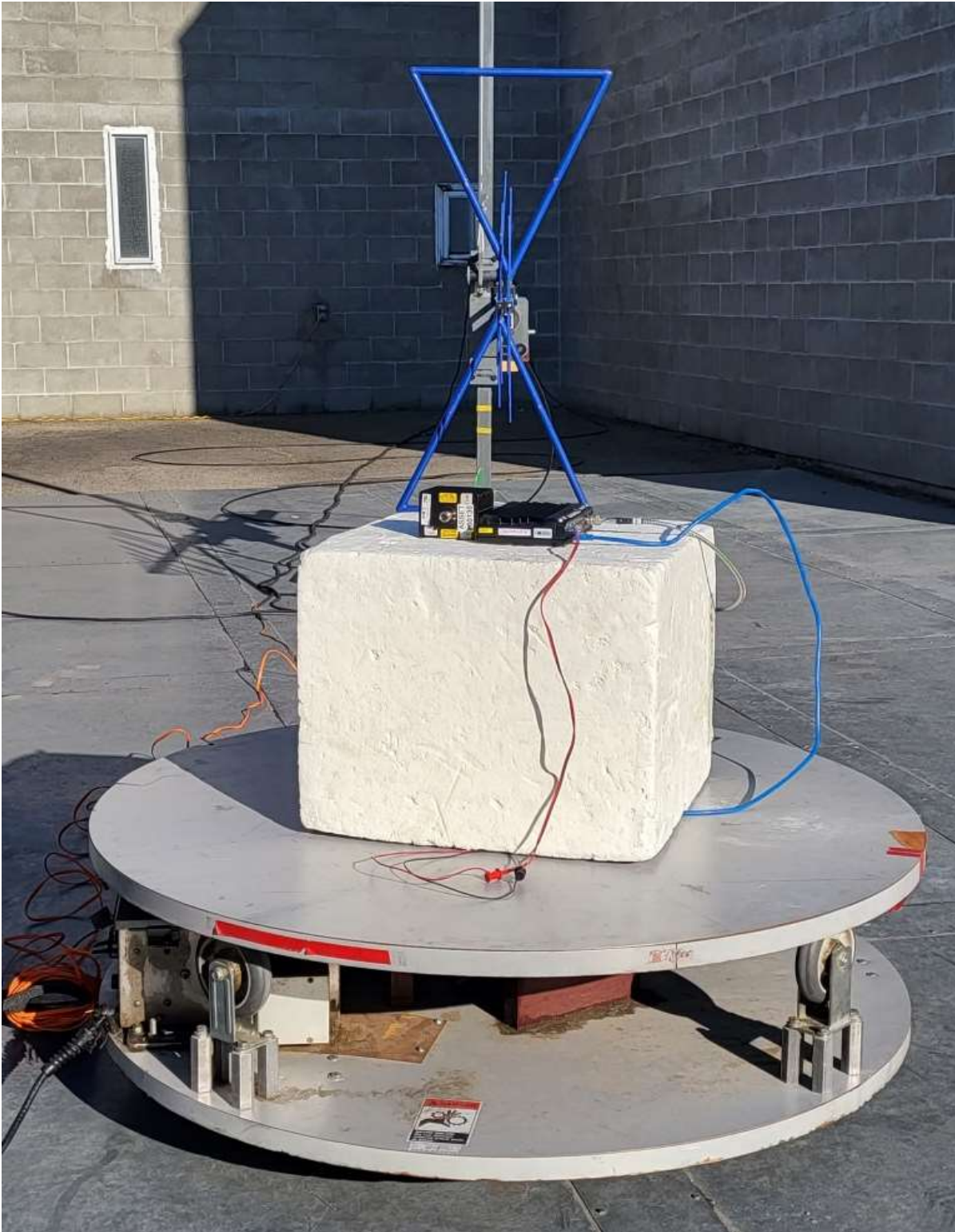
Figure E10.2 – Setup, Radiated Tx Measurements, 30-1000MHz
