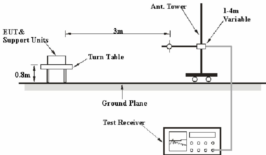
The radiated emission tests were performed in the 3 meters chamber A test site, using the setup accordance with the ANSI C63.4 - 2003. The specification used was the FCC Part 15.209 and FCC Part 15.239.
