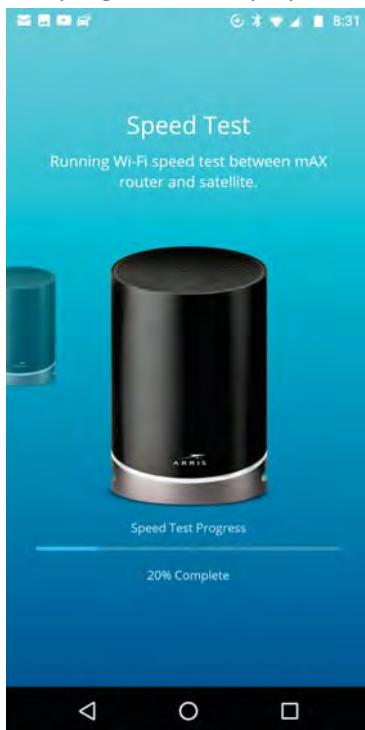
At the conclusion of the test, if the connection between the Router and Satellite is poor, you can choose to relocate the Satellite and tap **Test again**, or skip the test and tap **Continue** to continue with your mAX Satellite installation.
