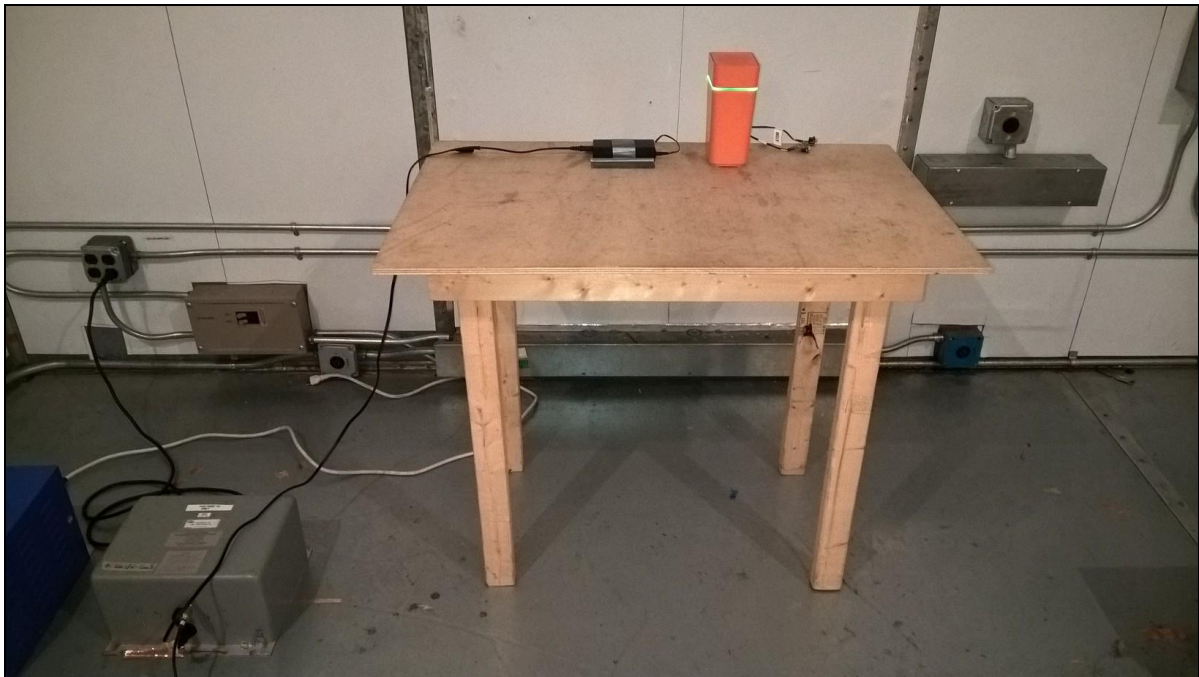
Photograph 3. Conducted Emissions, Test Setup
