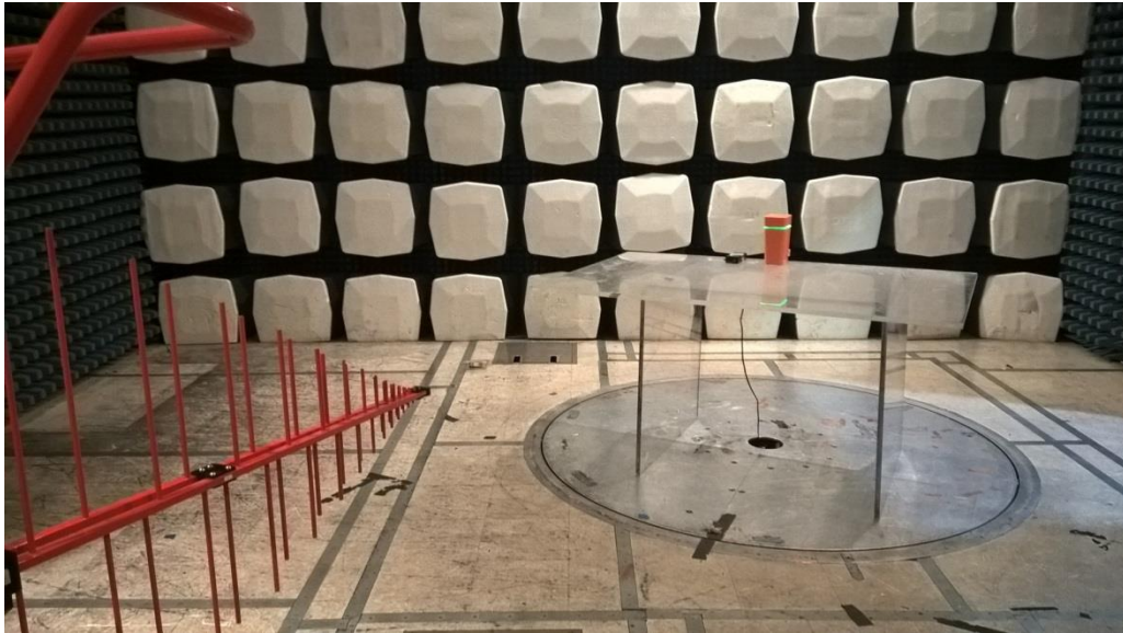
Photograph 2. Radiated Spurious Emissions, Test Setup below 1GHz
