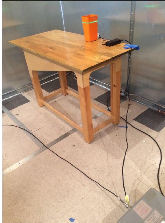
Photograph 1. Conducted Emissions, 15.207(a), Test Setup
