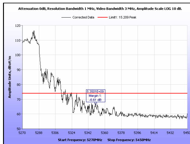
Plot 1263. Restricted Band Edge, 802.11ac 40 MHz, 5270 MHz, Peak, 8x8
