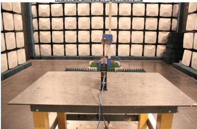
RADIATED EMISSION TEST 30MHz to 1G
