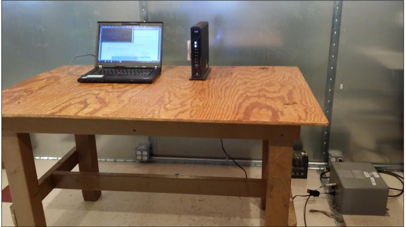
Photograph 1. Conducted Emissions, Test Setup
