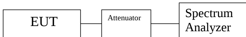
Figure 3. Power Output Test Setup
