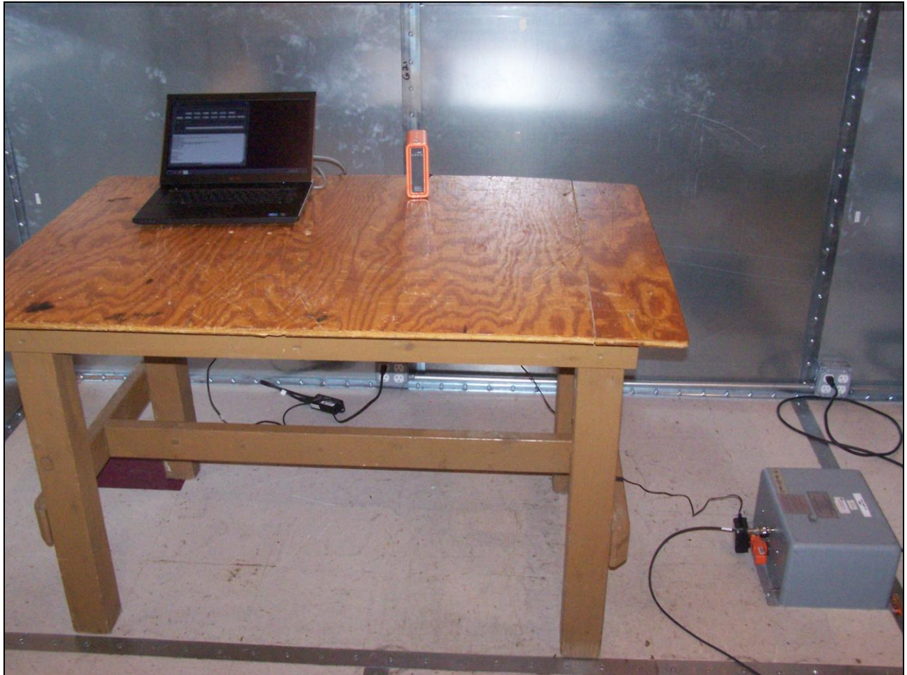
Photograph 2. Conducted Emissions, 15.207(a), Test Setup
