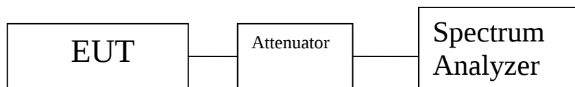
Figure 1. Block Diagram, Occupied Bandwidth Test Setup
