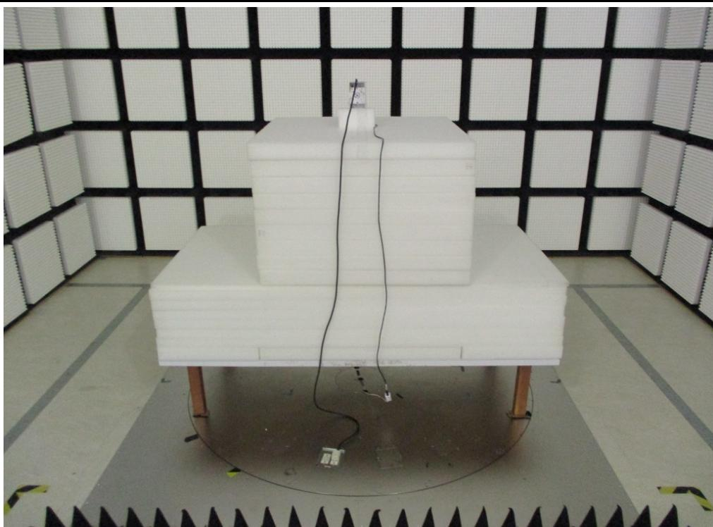
**Radiated Emission Above 1GHz Test**
