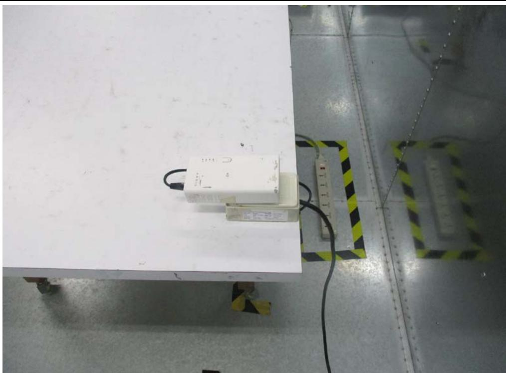
**Radiated Emission Below 1GHz Test**
