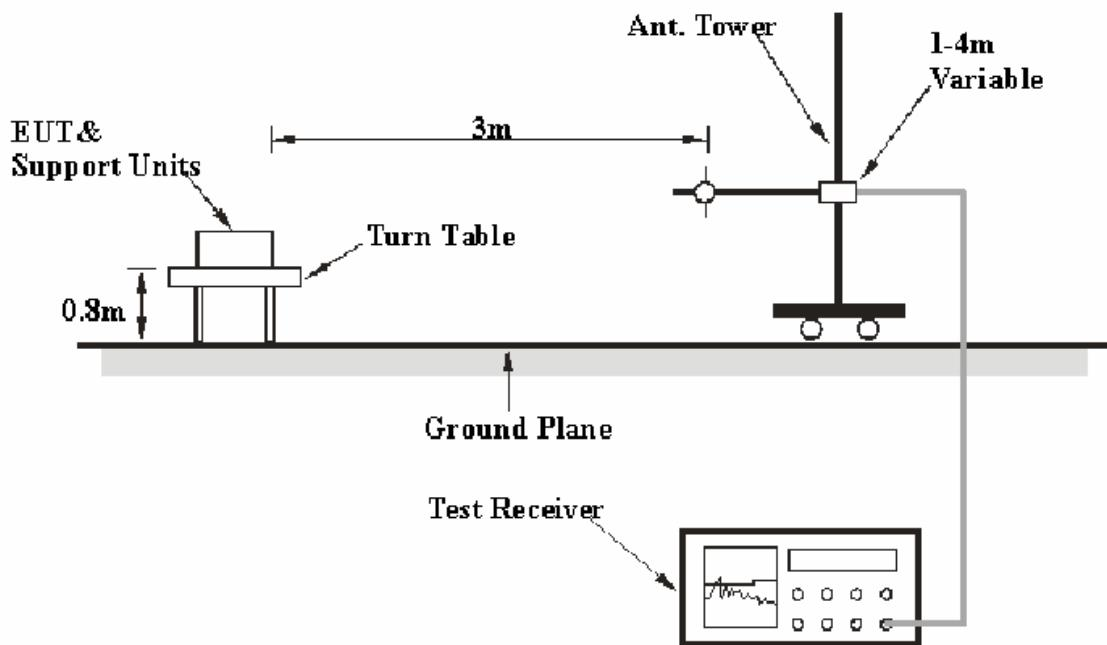
The radiated emission tests were performed in the 3-meter chamber A test site, using the setup accordance with the ANSI C63.4-2003. The specification used was the FCC Part 15.227 limits.
