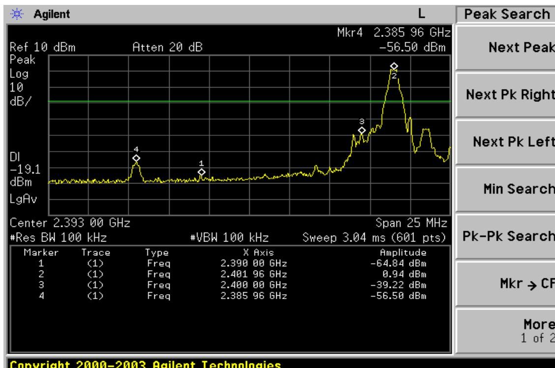
**Conducted Emission: Test Data CH-High**
