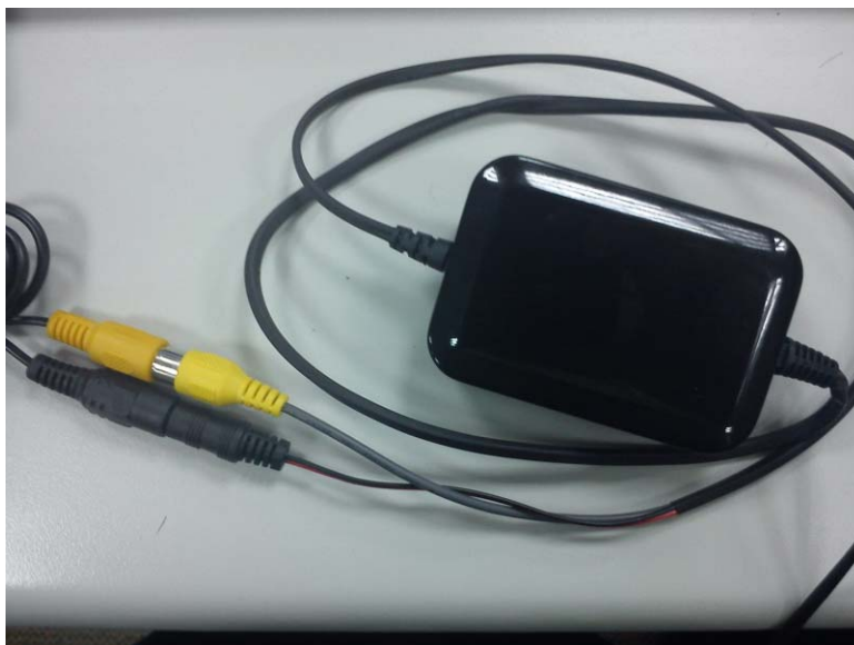
Connected camera's Video Out and Power in to transceiver.
