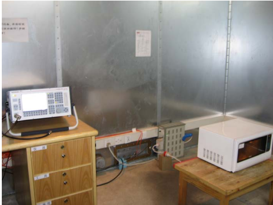
Conducted Emission Test Set-up
