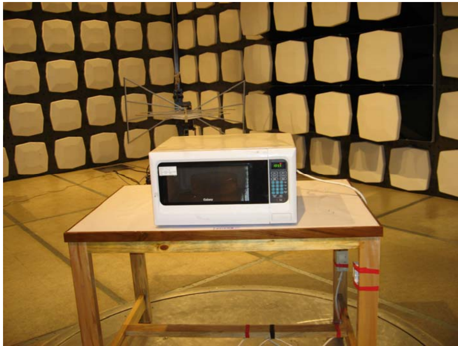
Radiated Emission Test Set-up (30~1000MHz)
