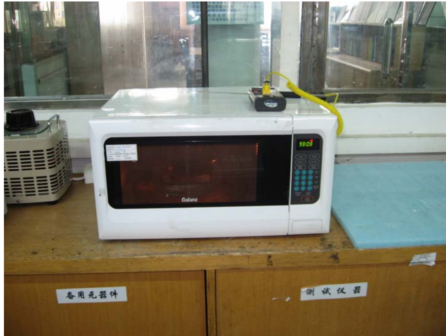
RF Output Power Test Set-Up
