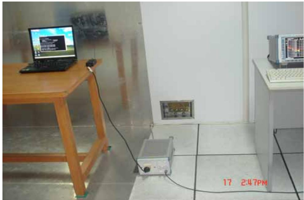
**Radiation Emission Test View For 30MHz-1000MHz**
