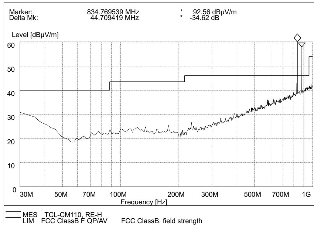
(Note: The marker points are the MS and BS transmitting frequencies which should be ignored.)
