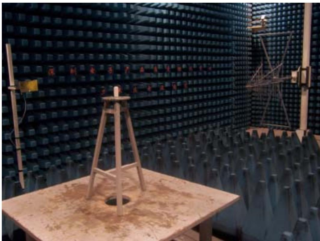
**5. Radiated RF Test (9 kHz~30 MHz)**
