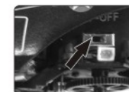
The 'ON/OFF' switch is located on the side of the fuselage.
