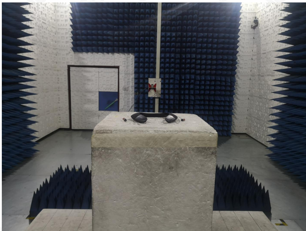
RADIATED EMISSION TEST SETUP ABOVE 1GHZ
