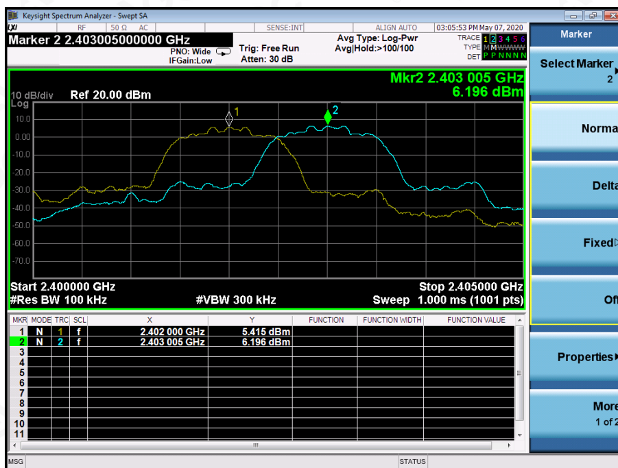
TEST PLOT FOR FREQUENCY SEPARATION
