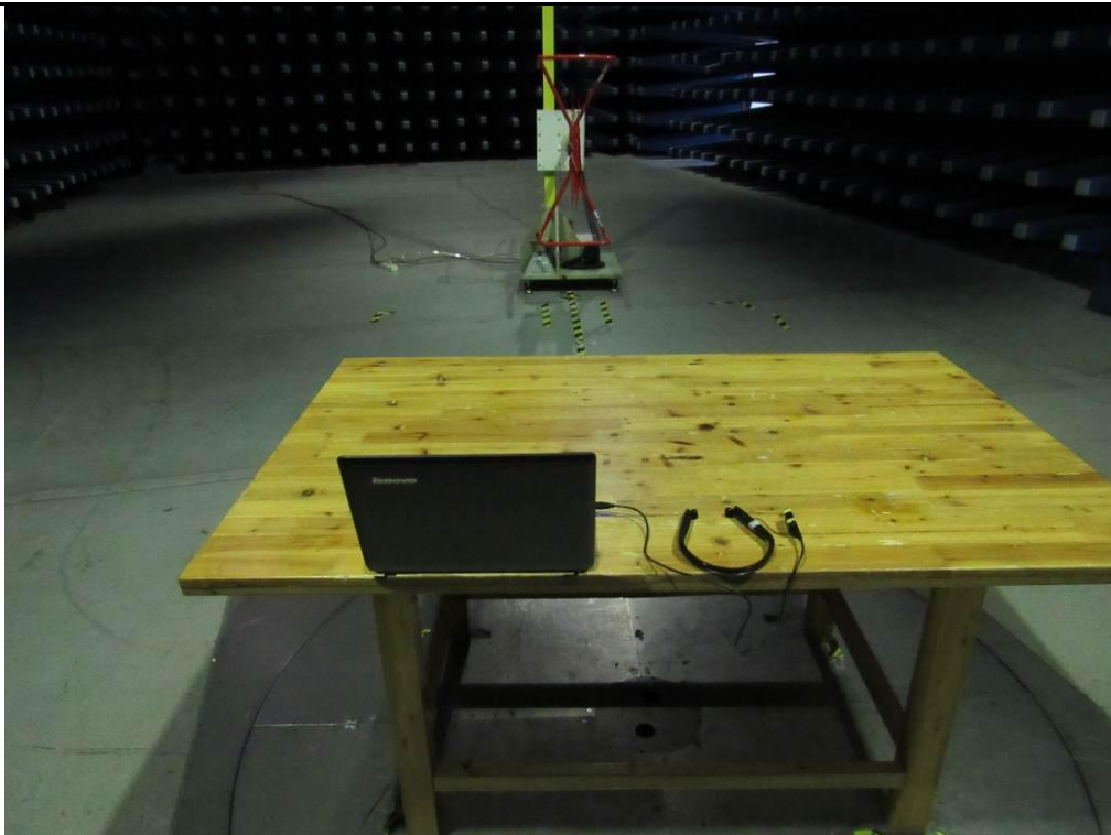
Radiated Spurious Emissions Test Setup Above 1GHz
