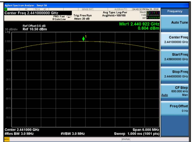
8DPSK Output power - Mid CH 2441
