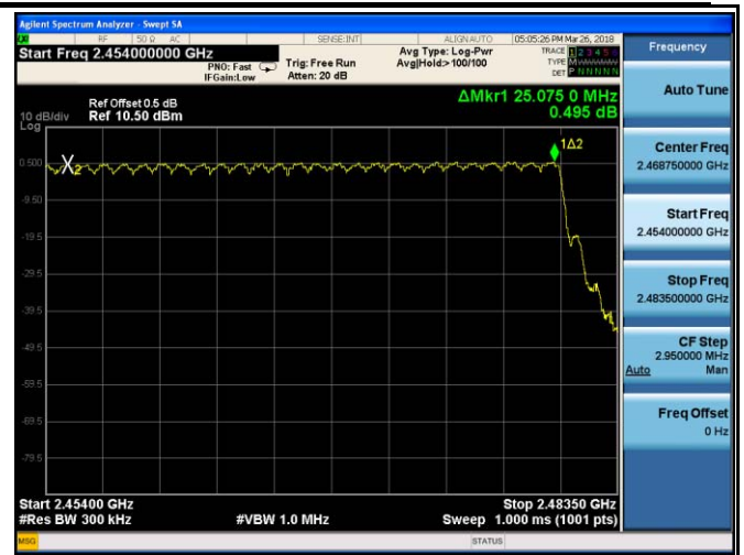
\pi/4 DQPSK Number of Hopping Channels - 3
