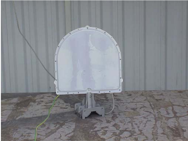
Photo # 1. Radiated emission test set up. Front side view.
