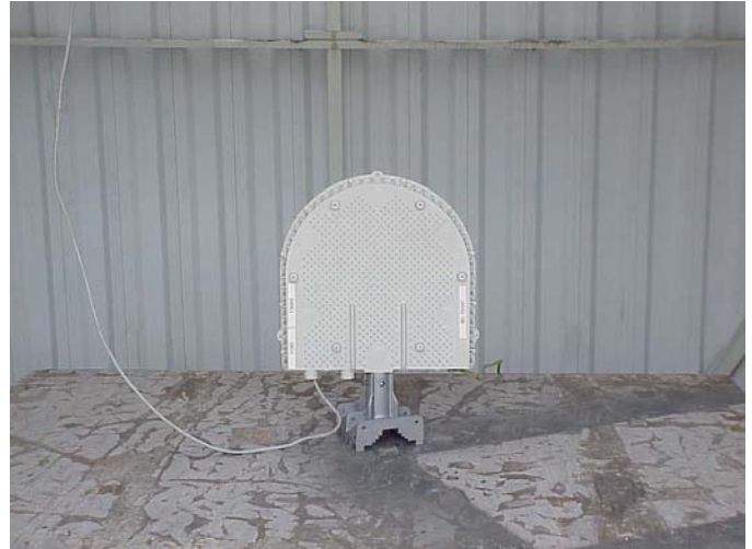
Photo # 2. Radiated emission test set up. Rear side view.
