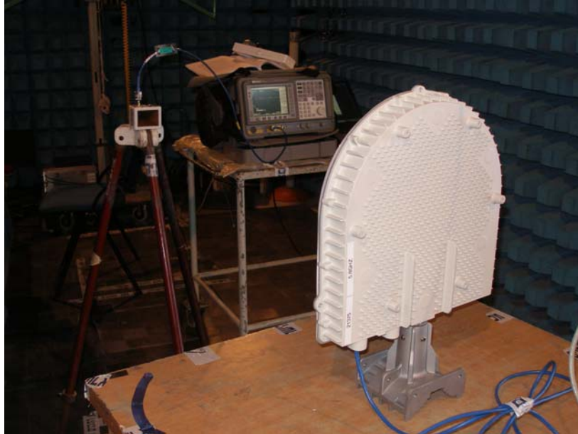
Photo # 5. Radiated emission test on Outdoor Radio Unit: spurious & restricted bands.
