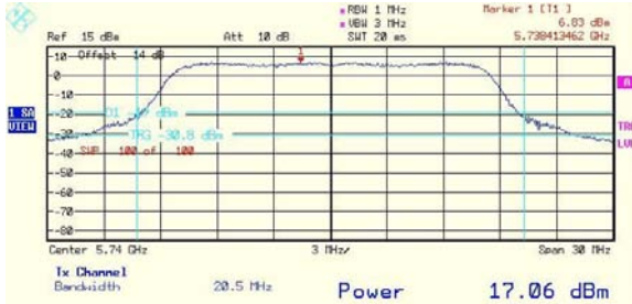
Plot # 52. Output 1 peak power. Lower frequency. 6Mbps rate.
