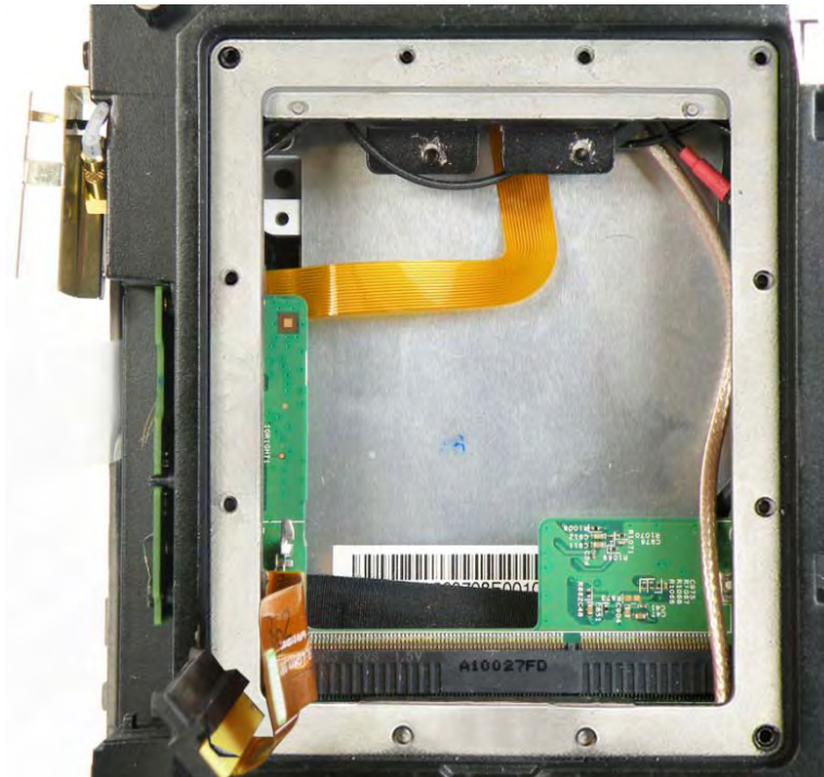
Figure 24. Internal Flexspace with the SSD and Flexboard Removed
