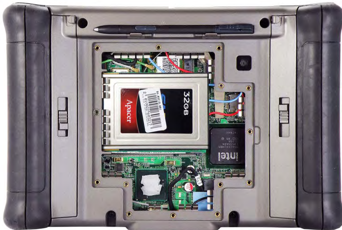
Figure 73. X7 Solid State Drive Location
