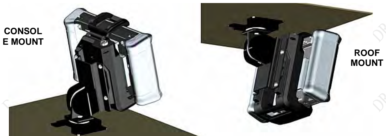
Figure 15. Examples of X7 Vehicle Dock Mounting Configurations
