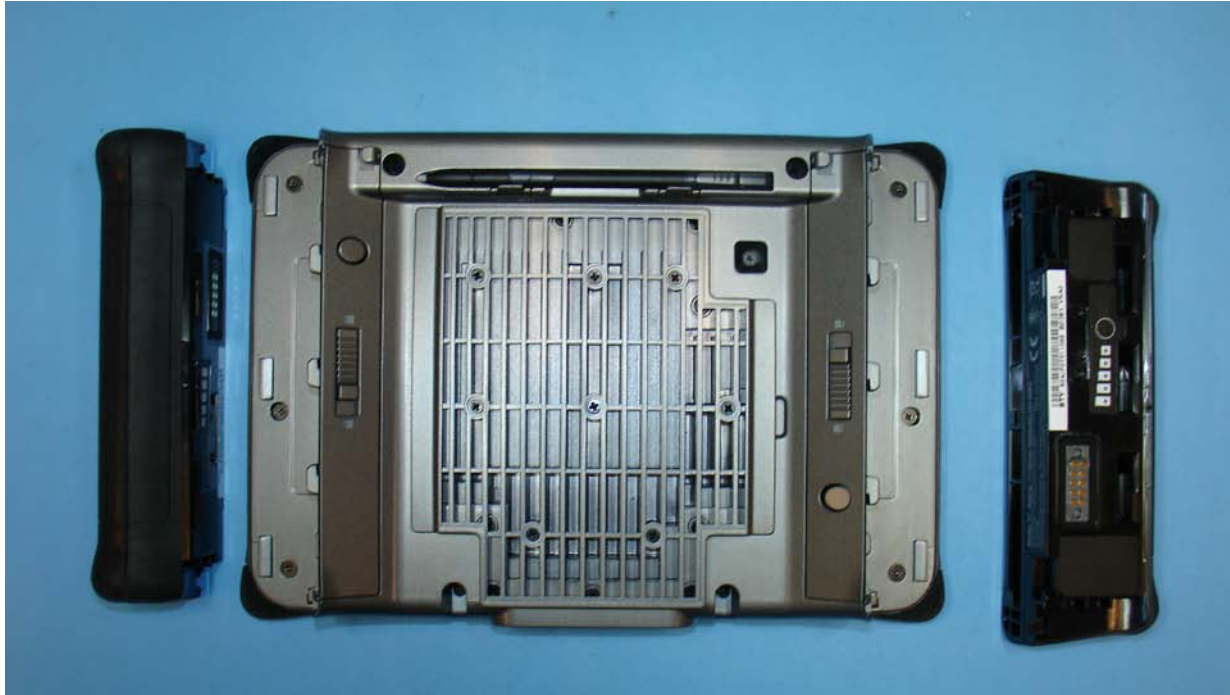
Figure 6 Armor X7 Back Side View, Batteries Removed
