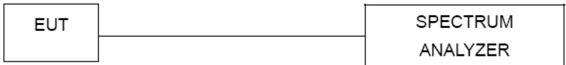
2. The bandwidth of the fundamental frequency was measure by spectrum analyser with 1MHz RBW and 1MHz VBW. The 20dB bandwidth is defined as the total spectrum the power of which is higher than peak power 20dB.
