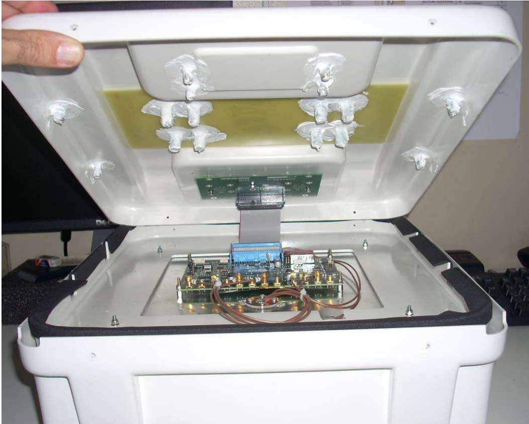
Fig. 1: Internal view of the antenna once the top cover has been unscrewed and lifted
